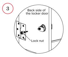
Place the lock nut, tighten the lock nut clockwise and make sure it is securely fastened but not too tight.
