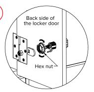
Insert the lock through door routing followed by the hex nut. Tighten the hex nut clockwise and make sure it is securely fastened.
