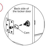
Insert the cam through the cylinder bolt and make sure the cam is facing towards the edge of the door.
